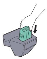
Insert the key counter securely into the key counter slot.
